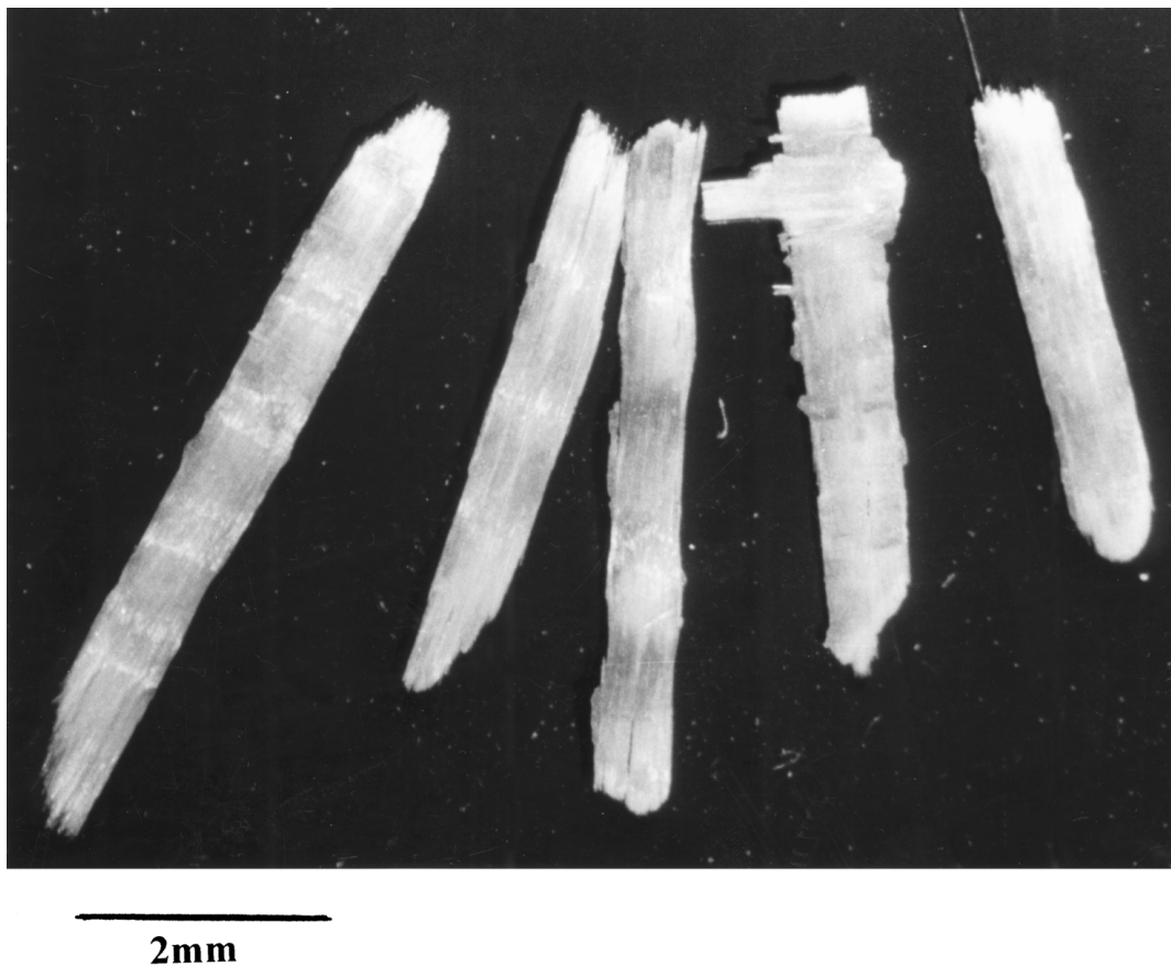
Figure 4 Fibre tows in 4 mm GWP feedstock.
